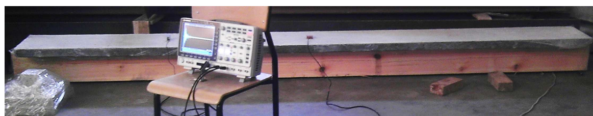
Fig. 6. The picture, horizontal projection and cross-section of the tested composite beam
